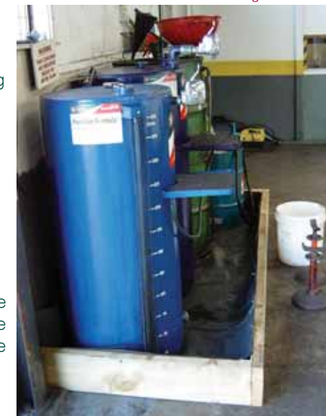
Oil store after new homemade 'bunding'
